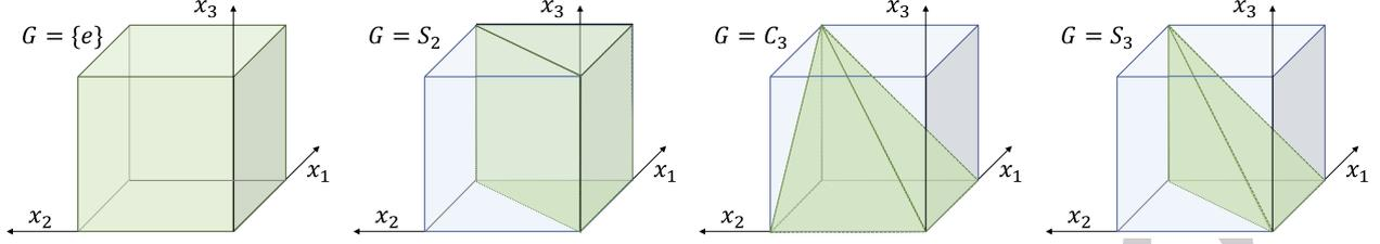
Figure 2: Example of quotient feature spaces with  $n = 3$ . (i) trivial group case ( $G = \{e\}$ ):  $\Delta_{\{e\}} = [0, 1]^3$ . (ii) symmetric group case ( $G = S_2$ ):  $\Delta_{S_2} = \{x \in [0, 1]^3 \mid x_1 \geq x_2\}$ . (iii) cyclic group case ( $G = C_3$ ):  $\Delta_{C_3} = \{x \in [0, 1]^3 \mid x_1 \geq x_2 \geq x_3\} \cup \{x \in [0, 1]^3 \mid x_1 \leq x_2 \leq x_3\}$ . (iv) symmetric group case ( $G = S_3$ ):  $\Delta_{S_3} = \{x \in [0, 1]^3 \mid x_1 \geq x_2 \geq x_3\}$ .
