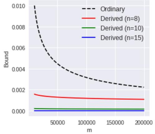
Figure 1: Order of the bound for the generalization gap against  $m$ . *Ordinary* (dashed line) denotes  $(1/\sqrt{m})$  without invariance, and *Derived* (colored lines) denote the bound  $(1/\sqrt{n!m^{2/n}})$  with  $n \in \{8, 10, 15\}$ . Regardless of the effect of  $m$ , the derived bound gets tight sharply as  $n$  increases.
