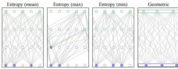
Figure 9: Optimal placements for six sensors for different algorithms. Entropy (max) selects also sensors within the area, while others favor sensors at the border.
