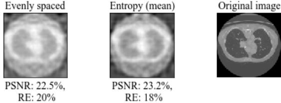
Figure 7: Means of the GP fit for nine sensor locations chosen using entropy (middle) and the even spacing typically used for CT scans (left). The true image (right) is reconstructed with comparable accuracy, with the proposed method here having slight edge.
