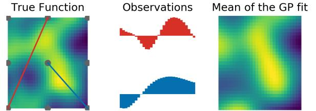
Figure 1: Solving a spatial inverse problem with line integral observations. **Left:** An unknown function is monitored by a collection of 9 sensors, each transmitting a signal that can be recorded by each of the other sensors. **Middle:** Illustration of two slices of the function along two example integration paths. **Right:** Mean estimate of the function, conditional on noisy observations of all 36 line integrals induced by the 9 sensors.
