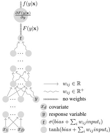
Figure 1: The graph representing Univariate Monotonic Neural Density Estimator computational structure. The last node symbolizes the operation of differentiating parameterized conditional distribution function  $F(y|\mathbf{x})$  with respect to the input  $y$ . Its output  $f(y|\mathbf{x})$  encodes the conditional density function. The legend explains the symbols used.
