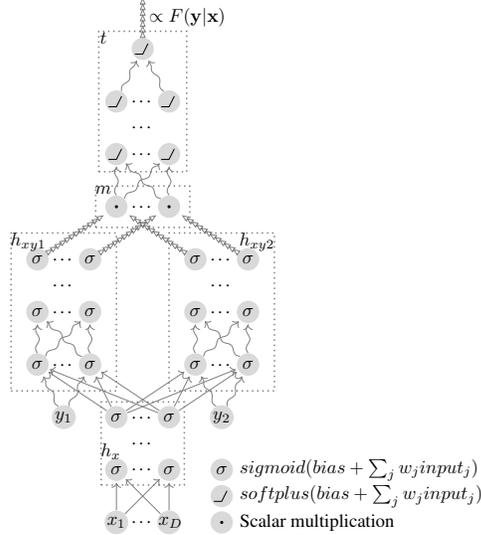
Figure 4: Graph of an “Unnormalized” Distribution Function of PUMONDE, Pure Monotonic Neural Density Estimator. It shows two response variables  $y_1, y_2$  and covariates  $\mathbf{x}$  transformed via computational graphs:  $h_x, h_{xy1}, h_{xy2}, m$  and  $t$ .
