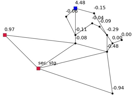
**Figure 5:** The electrical grid and (optimal) power generation for the optimal power flow problem on the IEEE 14 Bus Test Case. Red vertices are generators: a positive number indicates the optimal power generation, while “sec. stg.” denotes an uncontrolled generator. The blue vertex is a (stochastic) renewable generator: its mean available (wind) power is shown above it. Other vertices are loads: their (nonpositive) demanded powers are shown above them.
